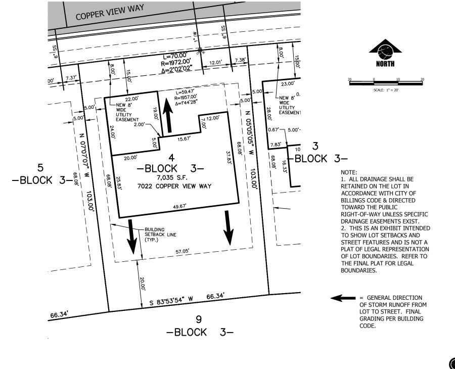
P:\96012\_00\_HOUSE\_LAYOUTS\COPPER RIDGE SEVENTH\16064\_03\_HOUSE LAYOUTS.dwg, 10/15/2018 2:25:03 PM, DWG To PDF.pc3
