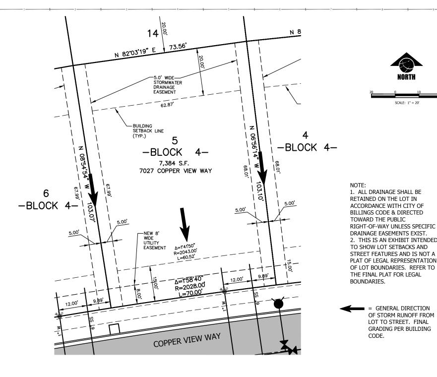
1. ALL DRAINAGE SHALL BE RETAINED ON THE LOT IN ACCORDANCE WITH CITY OF **BILLINGS CODE & DIRECTED** TOWARD THE PUBLIC **RIGHT-OF-WAY UNLESS SPECIFIC** DRAINAGE EASEMENTS EXIST. 2. THIS IS AN EXHIBIT INTENDED TO SHOW LOT SETBACKS AND STREET FEATURES AND IS NOT A
